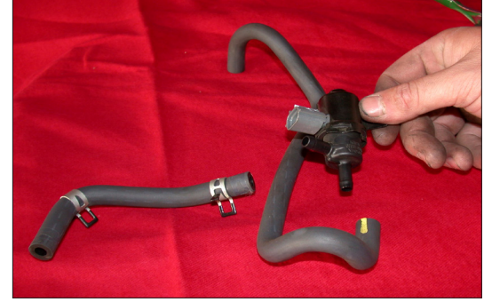
23. Remove the two vent hoses from the EVAP OBD canister closed valve as shown.
