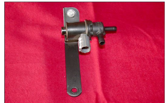
24. Secure the EVAP OBD canister closed valve to the provided angle bracket using the provided hardware as shown.
