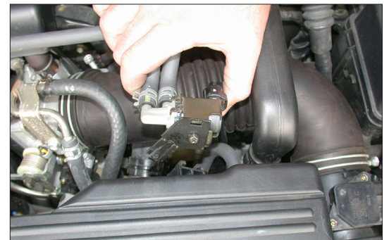
7. Unclip the PWM vacuum switching valve from the rear of the air cleaner assembly as shown.
