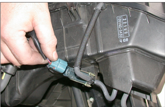
14. Disconnect the vacuum switching valve electrical connection as shown.
