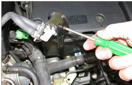
19. Remove the stock bracket from the PWM vacuum switching valve as shown.
