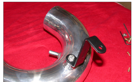
26. Secure the "Z" bracket to the threaded boss on the Typhoon intake tube using the provided hardware as shown. NOTE: Before installing the "Z" bracket, inspect the inside of the tube for any debris, then clean the inside out with water and a towel. Inspect the tube one more time before proceeding to the next step.
