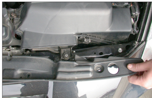
4. Remove the radiator core support cover as shown.
