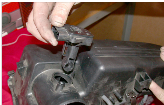
20. Remove the mass air sensor from the air cleaner assembly as shown.
