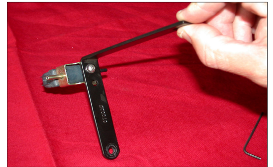
25. Secure the vacuum switching valve to the provided "L" bracket using the provided hardware as shown.
