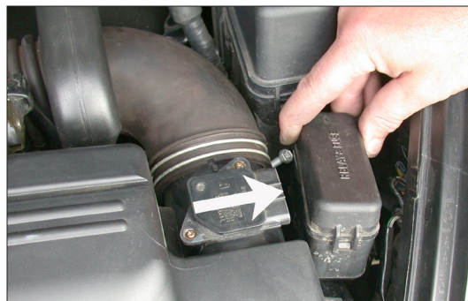
5. Unclip the relay and fuse box and move it out of the way as shown.
