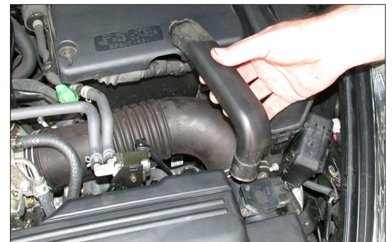
8. Pull firmly to remove the computer fresh air tube as shown.
