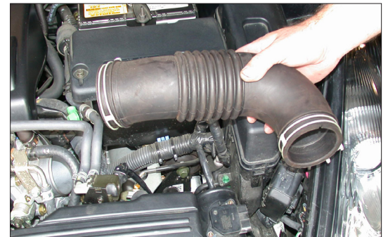
9. Loosen the hose clamps on the stock intake tube, then, remove the stock intake tube as shown.
