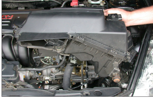
17. Remove the complete air cleaner assembly as shown.
